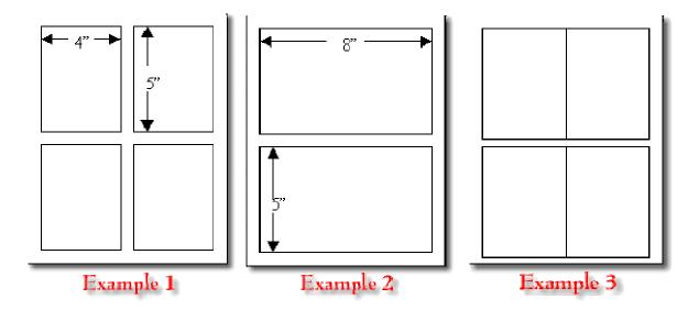
In Example 2 there are two shapes cut into a die, each shape being  $8" \times 5"$ . Each shape therefore has 26 lineal inches (8"+8"+5"+5"). There are two shapes on the die for a total of 52".
